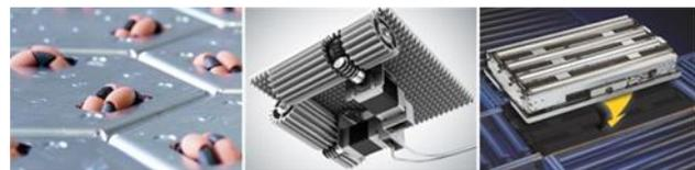
*Figure 1. Small-scaled modular conveyor systems: Celluveyor [UTF10, UTF16], Motion Cube [Fes15] and Magic Carpet [Ito16]*
