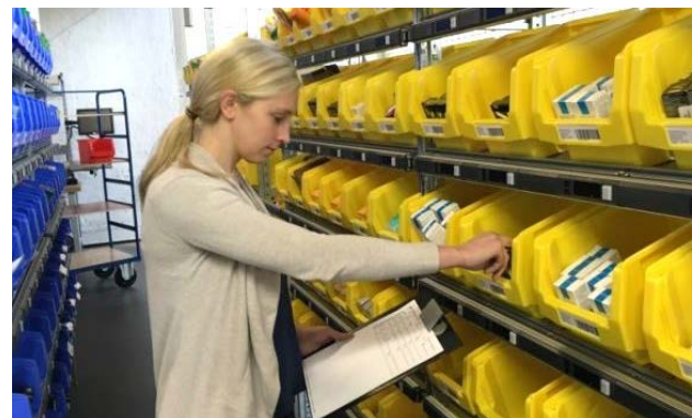
Figure 3. Pick-by-line with physical list
