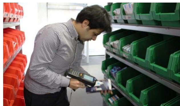
Figure 4. Pick-by-scan with handheld barcode scanner
