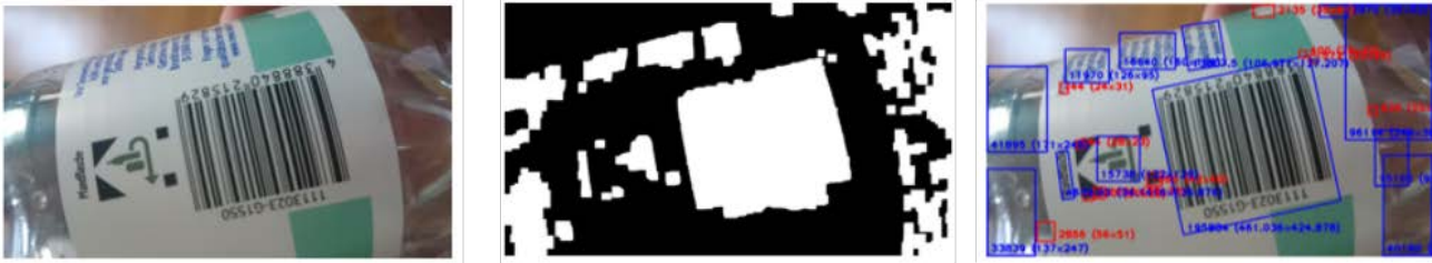
Figure 2. Example of the pre-processing for the barcode detection. Only the detected candidate regions are evaluated in order to speed-up the processing.
