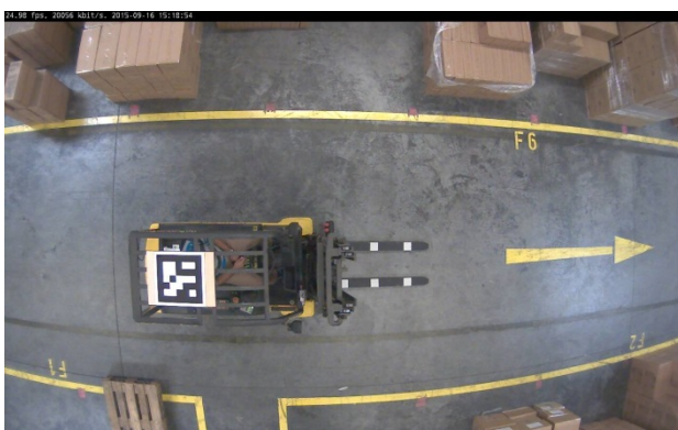
Figure 4. Forklift with ArUco matrix code on its top and a color pattern on the fork
