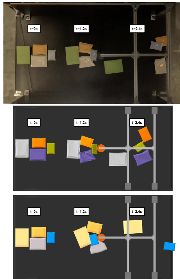
Figure 11. Representative obstacle-passage sequence comparing the experiment with the shell- and volume-based MFBD models at selected time instances.
