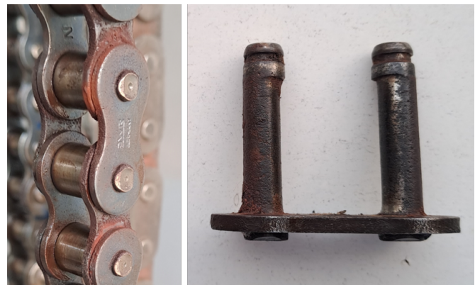
Figure 1: Results of dry operation of a roller chain. Tribocorrosion with rust powder on the left, excessive wear on the right
