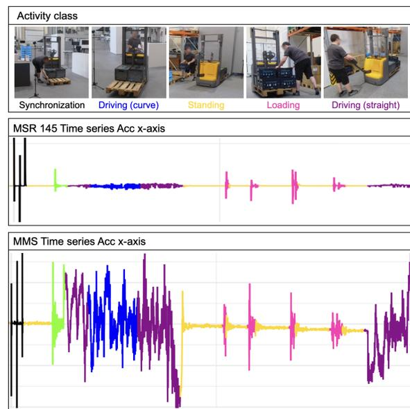
Figure 5: Excerpt of a scenario and comparison of the time series to video frames
