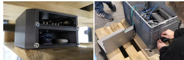
Figure 4: 3D printed pallet block containing the sensors (left) and power supply container with cable management (right)
