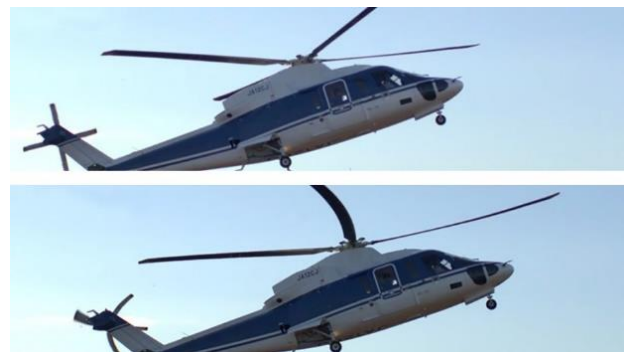
Figure 7 Global shutter(above) and Rolling shutter(below) [32]
