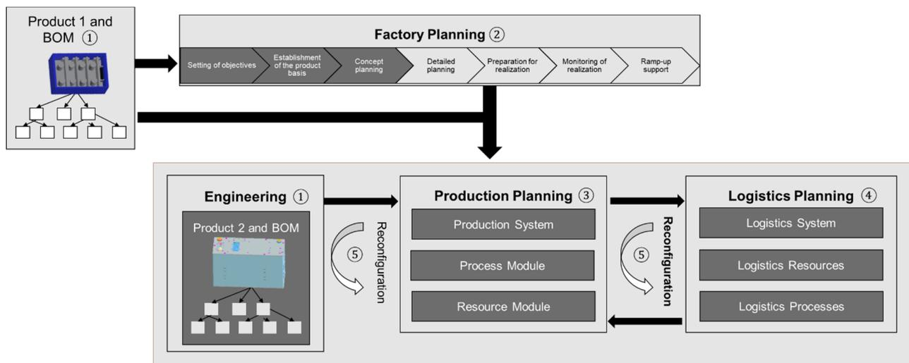
Figure 4. Approach for an integral factory, production, and logistics planning and reconfiguration.
