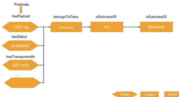
Figure 14. KG of the AMR based on [76]
