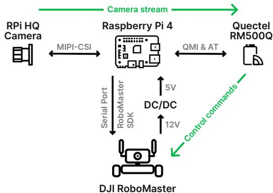
Figure 3: System architecture of the ground-bound AGV.
