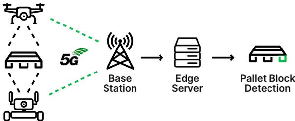
Figure 5: System architecture for the mobile re-identification of industrial entities.
