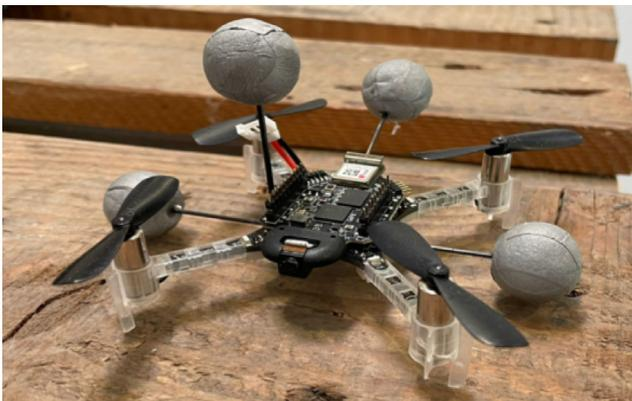
Figure 2: The aerial AGV, using a Crazyflie as its platform.
