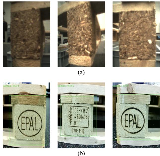
Figure 4: Images automatically recorded by the aerial AGV (a) and the ground-bound AGV (b) using YOLO to detect the three pallet blocks of interest.
