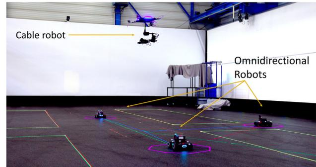
Figure 10. The technical setup for 3D network management in intralogistics, the cable robot is utilized as the relay node to enhance the coverage of omnidirectional robots.
