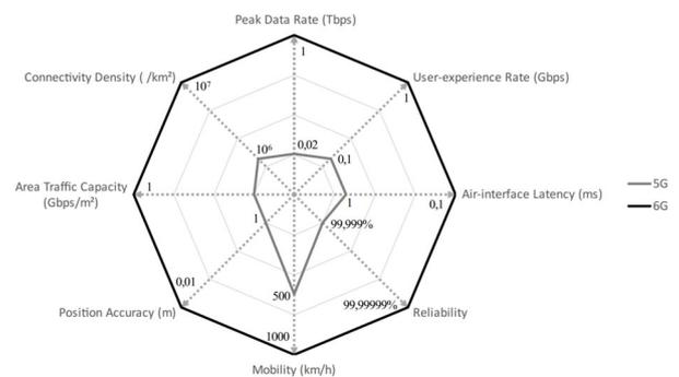
Figure 1. KPI's comparison of 6G and 5G technology, adapted from [16]–[18]
