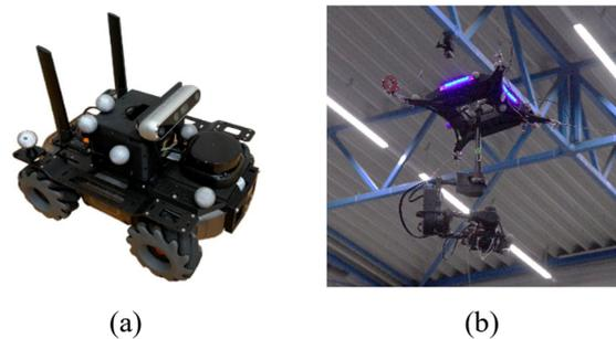
Figure 3. (a) Omnidirectional robot platform (b) Cable robot platform
