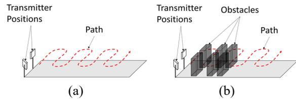
Figure 9. The illustration for the measurement scenario: (a). reference measurement with empty test field. (b). measurement with obstacles.
