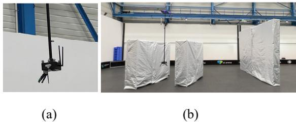
Figure 8. The technical setup for 3D REM: (a). 5G receiver on cable robot as data collector. (b). Measurement setup scenario using heavy-duty shelves.
