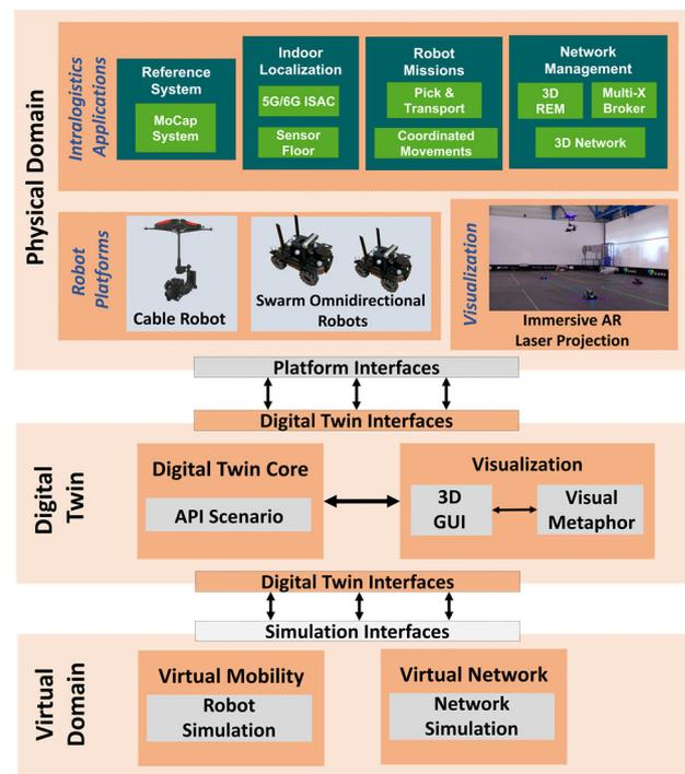
Figure 7. The proposed digital network twin architecture
