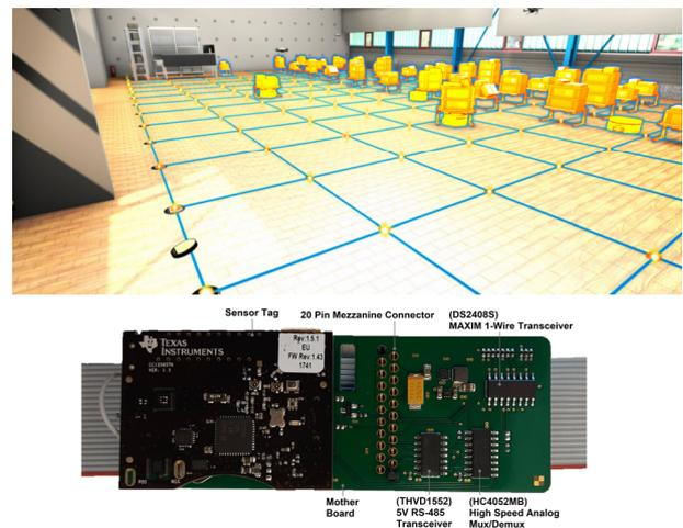
Figure 6. Rendered picture of the placement of Sensor Floor nodes and the implementation of a node using CC1350 SensorTag and extension board.
