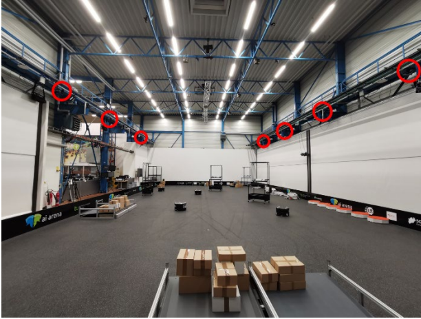
Fig. 3: Camera system installed at our research facility. Locations for seven of the eight installed cameras are circled in red.
