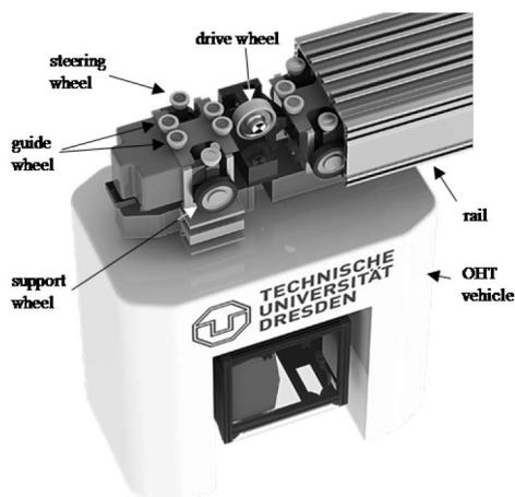
The long-term goal of our research is to inspect all the mentioned components automatically. For this paper, we will focus on measurements and analysis of the driving wheel although the subsequently presented approach is supposed to be applicable for the other mentioned wheels (and OHT-manufactures), too.
